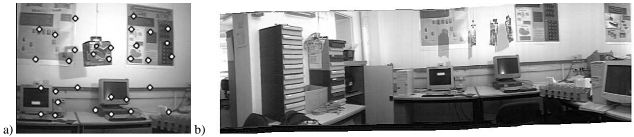
Figure 4. Mosaicing examples. a) Point selected for motion computation. Four of the thirty points are located on the moving pendulum. b) Panoramic image that was created while a pendulum was swinging. The alignment was not affected by the outliers.
